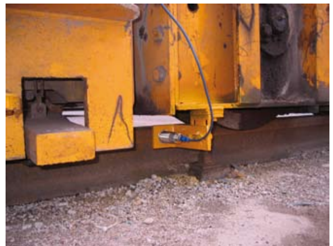
Contact between the wheel flanges and the rails is prevented. The accuracy of the signals from the four ultrasonic sensors is vital to the operation.
