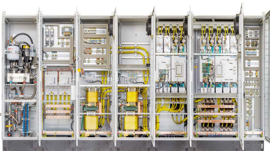
Complete 1.1MW cabinet with water-to-water cooling. Cabinet sections from left to right : 1) Cooling 2) Main switch 3) and 4) LCL filter 5) AFR with 4 PEBBs 6) VSI with 5 PEBBs 7) Aux section.
