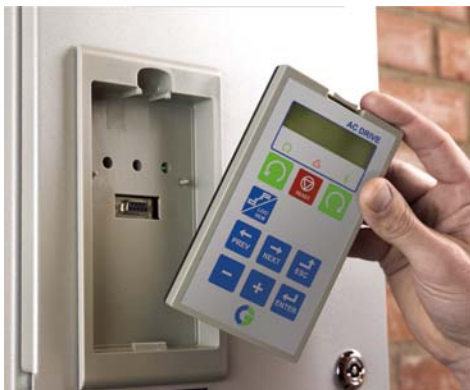
Fig. 1 When you remove the blank panel or control panel you will be able to connect the HCP.
